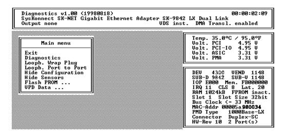
Fig. 11. Simultaneous display of sensor and configuration data
